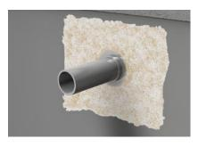
5. Quartz sand After curing, apply the 2nd layer of ASODUR-SG3-thix using a rolling technique and scatter quartz sand 0.5 -1.0 mm on the primer while still fresh.
