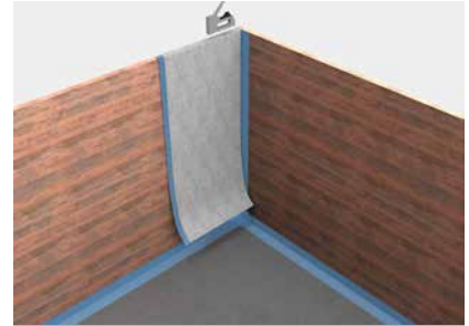
3. Tack AQUAFIN-WM12 on top and guide it down, starting with the corner.
