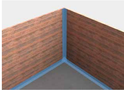
2. Continue the corner with PVC sheeting.
