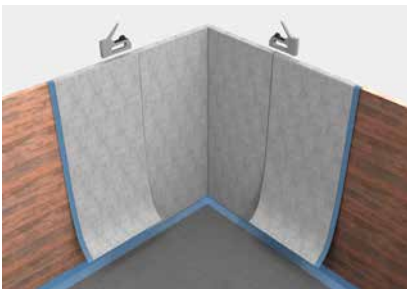
4. Weld or glue web overlaps together.
