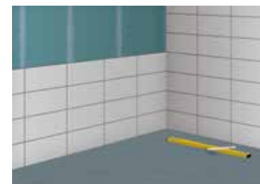
9 Setting out the floor
