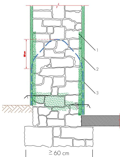
Perform the renovation until at least 80 cm above moisture level or recognizable salt infestation
