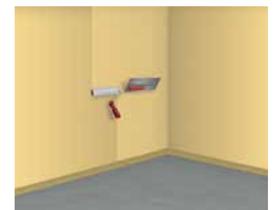
8 Application of the second coat of waterproofing membrane
