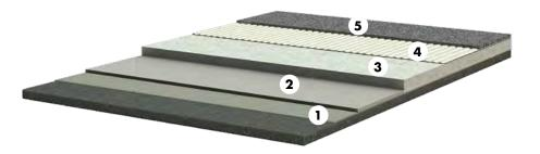
In order to install tiles on poured asphalt, this must be of minimum quality AS-IC 10 and have a minimum thickness of 25 mm. The asphalt screed must have from 10 - 15 mm movement joints against adjoining building components, which are to be brought through to the final floor surface. If the screed is newly installed, ensure that it is fully covered with quartz sand. If this is not the
