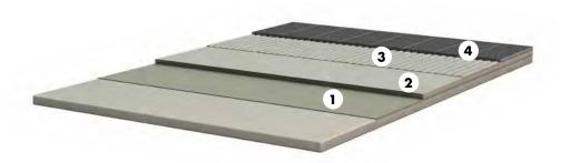
Direct contact between cement-based tile adhesives and magnesite screeds leads to the destruction of the magnesite screed due to a chemical reaction known as 'magnesite pouring'. Moisture pressure from the rear of the substrate must be prevented through appropriate measures. Mechanically roughen the
