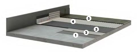
In commercially used wet areas, a particular type of waterproofing is necessary due to the large amounts of water present. The use of bonded waterproof systems (including the bedding mortar for the tiles and boards) protects all building components against moisture.
