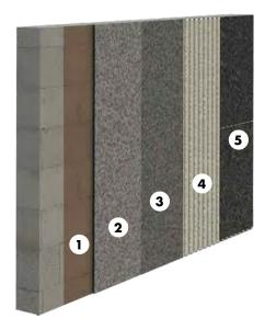
All plasters beneath ceramic tiles or natural stone must be struck off tightly with a straight edge. The surface must remain rough and may not be smoothened or felt boarded. To enable an orderly tile installation, increased requirements for flatness of the plaster should be contractually stipulated.
