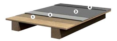
Wood substrates must be clean, dry and load bearing. Chipboard must be laid bonded, screwed and glued. Faulty wood/board substrates must be replaced, loose floor boards must be professionally fixed (e.g. screws, etc.). Seal joints between boards, planks. Please refer to our
