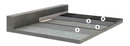
The selection of a suitable system is very important for the sound  $% \left( x\right) =\left( x\right) +\left( x\right)$ installation of stone and ceramic on balconies and terraces. Due to different expansion of the materials used, stresses occur
