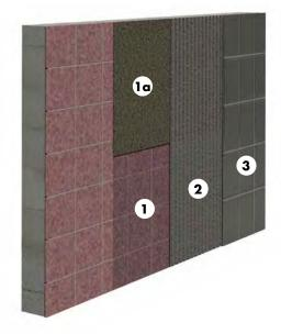
The existing tiled finish must be firm and load bearing. Remove loose areas and level with MGIII cement-based mortar. The substrate must be cleaned and all adhesion inhibiting components, such as lime, grease, dirt, etc., must be removed.
