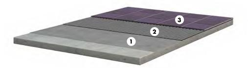
Cotto is an elaborate production process from fired clay material with a quite particular charm. Particular care and practical knowledge is needed to install cotto. Installation on damp screeds can quickly lead to efflorescence. In order to keep drying times short, a thin- or medium-bed adhesive with rapid crystalline binding of the mixing water should be used. Before grouting, it is recommended to impregnate the dry tiles in order to ease
