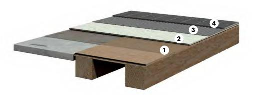
When carrying out building conversions or renovation work, critical substrates are often encountered. They have to be levelled, de-coupled and impact sound transmission reduced before installing tiles. Here the impact sound deadening and de-coupling board STEPBOARD can be used. To reliably prevent height differences, it is recommended that existing cracks in the substrate are adhesively sealed, e.g. ASODUR-K900.
