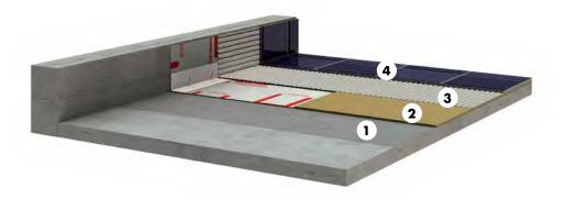
Due to the grouting, tiled and board finishes are not water tight. Therefore, in areas exposed to water, they require waterproofing in order to protect the substrate against moisture.
