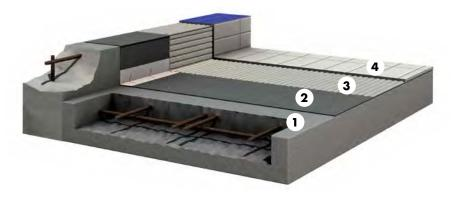
In order to impede the penetration of bathing water in the levelling layer and the concrete construction of swimming pools, suitable and approved waterproofing systems bonded with the tiled finish are used.
