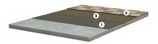
By using the highly flexible tile adhesive UNIFIX-S3/UNIFIX-S3-fast it is possible to lay tiles on a 'green' cement-based screed as soon as it is able to bear foot traffic. When laying tiles on 'green' cement-based screed the not yet completed setting process of the screed and the resultant low strength must be taken into account.
