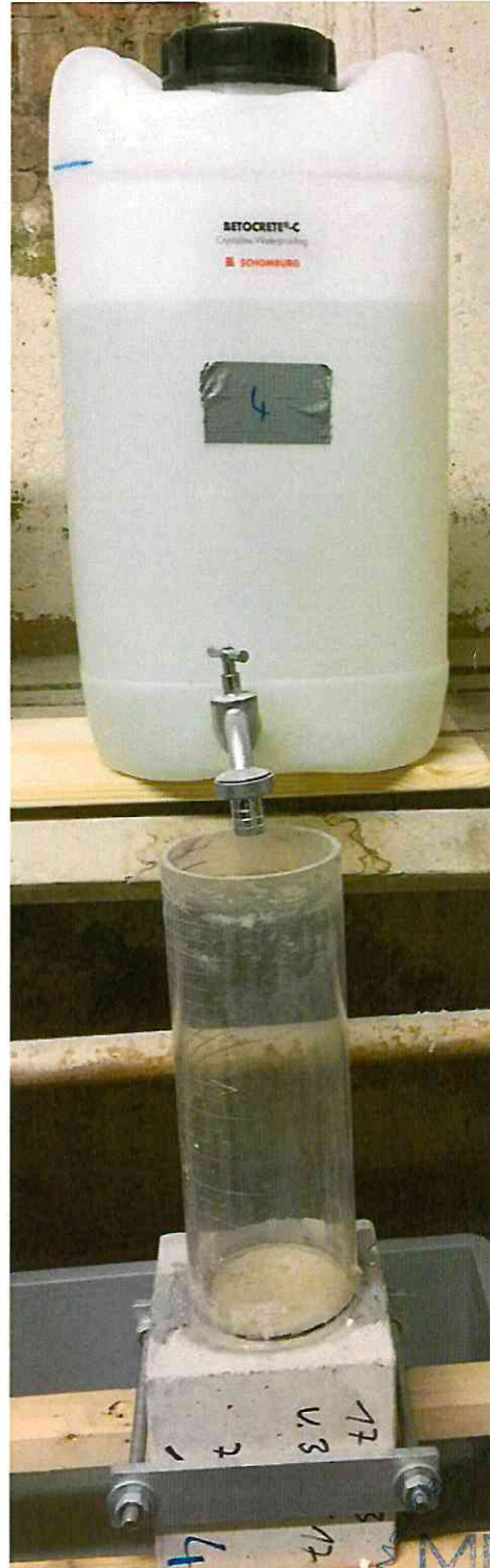
Appendix A-3: Special test setup for testing the passage of the amount of water through the crack
