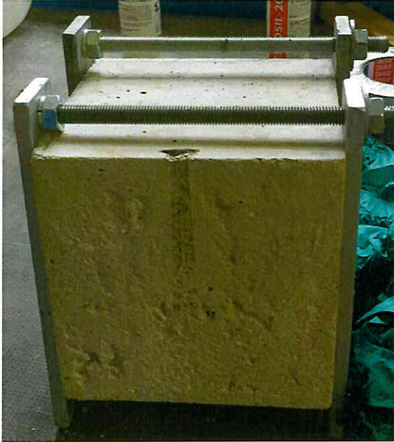
Appendix A-1: Sample before crack initiation
