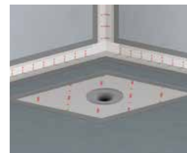
7 Bonding ASO®-Joint-Sleeve-Floor in the first coat of the waterproof membrane
