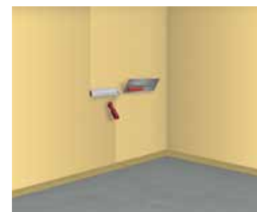
7 Application of the second coat of waterproofing membrane
