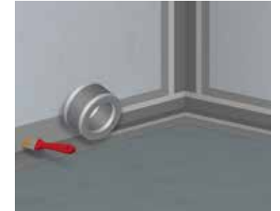
4 Bonding the ASO®-DB-Standard into the first coat of the waterproofing membrane
