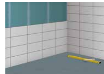
9 Setting out the floor
