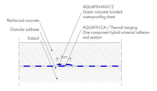
Overlap area thermal merging / bonding >4cm
