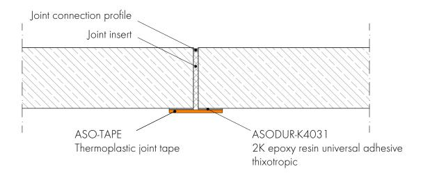
Overlap area ASO-TAPE / watertight concrete >5cm up to 2bar and >20cm with water pressure 2 to 5bar
