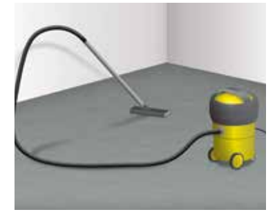
2 Cleaning the substrate
