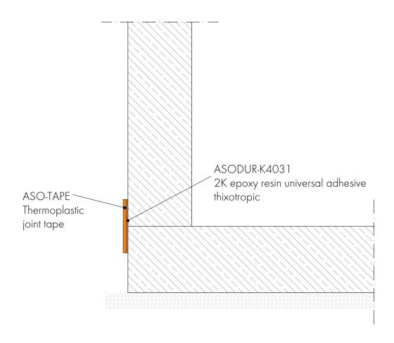
Overlap area ASO-TAPE / watertight concrete >5cm up to 2bar and >20cm with water pressure 2 to 5bar
